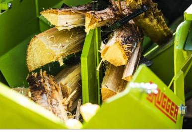
If a log lifter or chain conveyor is used, logs longer than 5m can be processed. In the basic version of the machine, the length is 2m.
