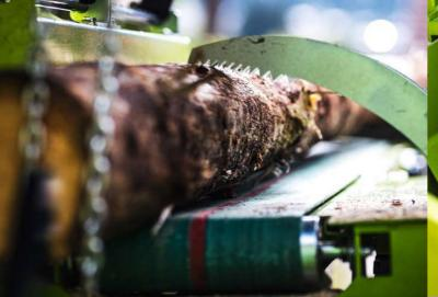
The length of the logs can be adjusted continuously from 15 up to 55 cm.
